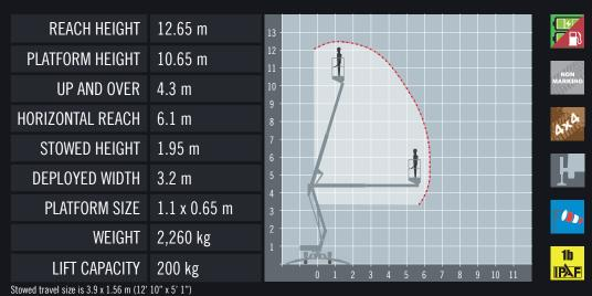
HYBRID POWERED Diesel and Battery power for flexibility
